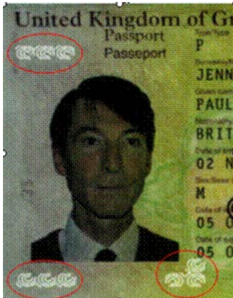
Laserperforerede strukturer/figurer: Destri Perf®
