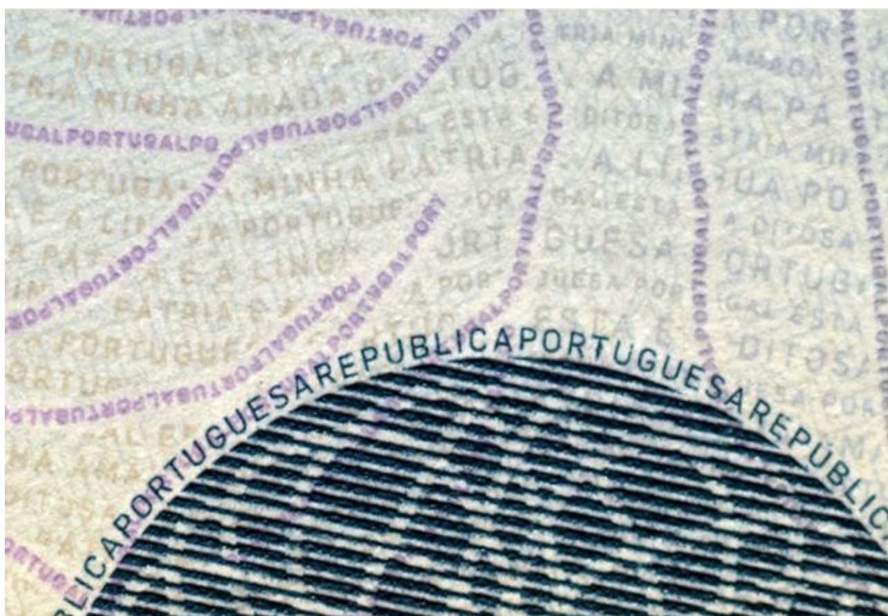
Miniprint (the blue text) and microprint (smaller purple letters)
