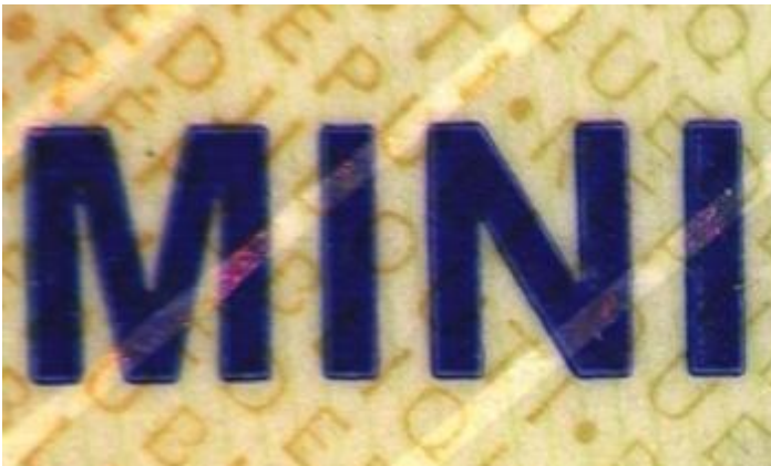
Flexo printing on → laminate
