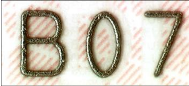
Tactile laser engraving of the numbering
