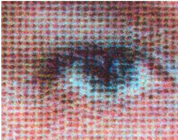
Biodata & photo integration technique: laser printing
