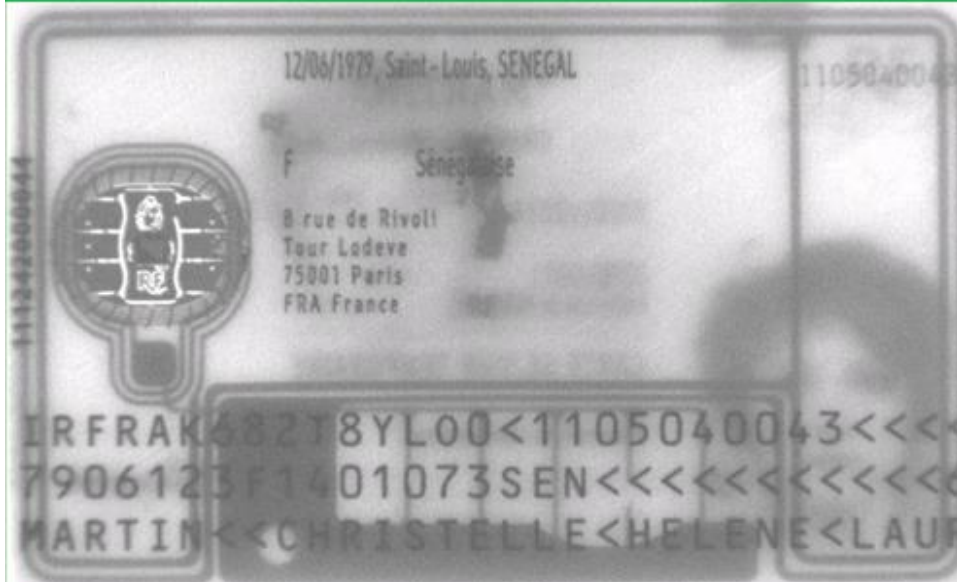
Contact chip and contactless chip and specially formed loop antenna in the polycarbonate card are visible under ➡ transmitted light .
