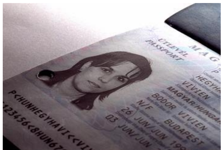
Laser-engraved integrated image
