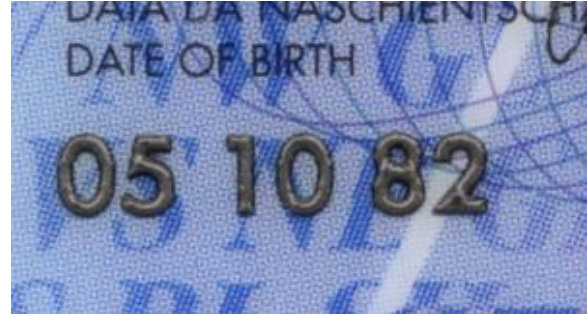
Tactile laser engraving of the date of birth
