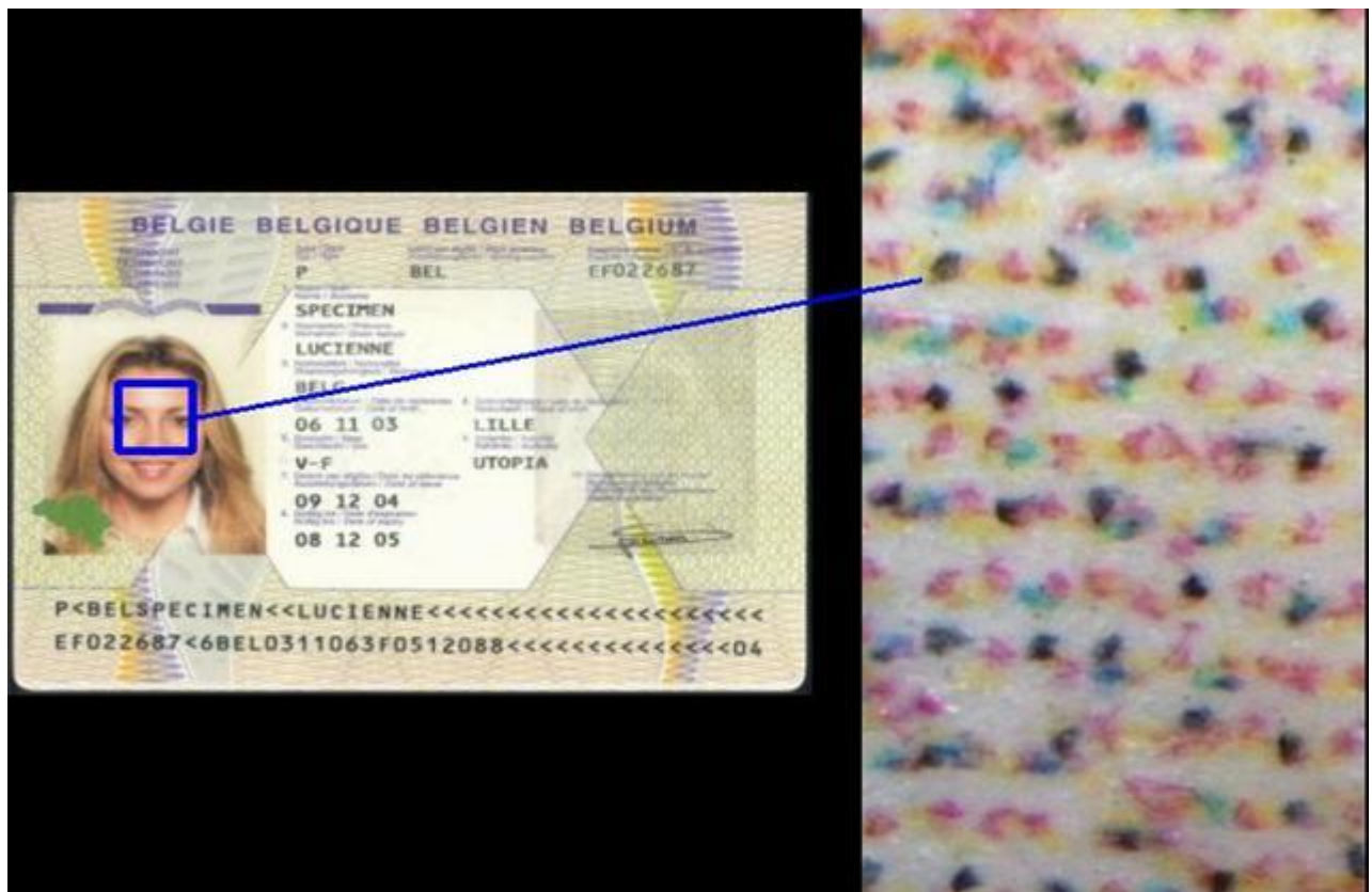
Biodata & photo integration with inkjet printing
