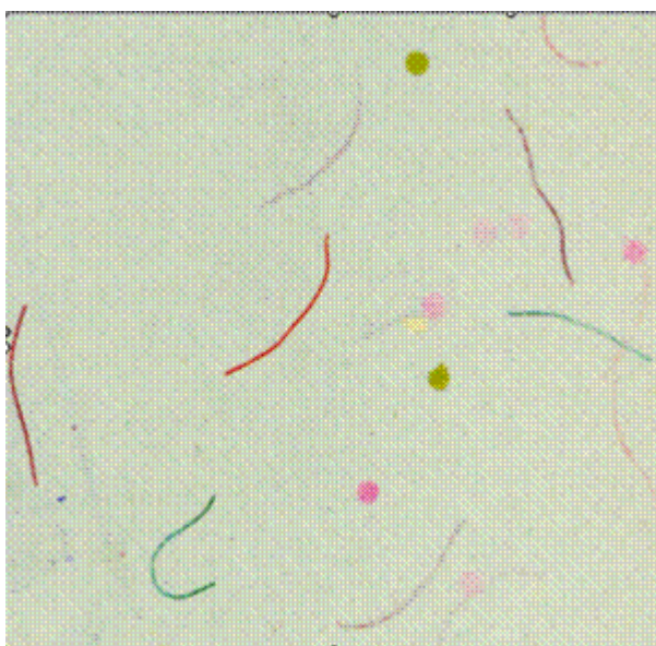
Coloured planchettes and fibres
