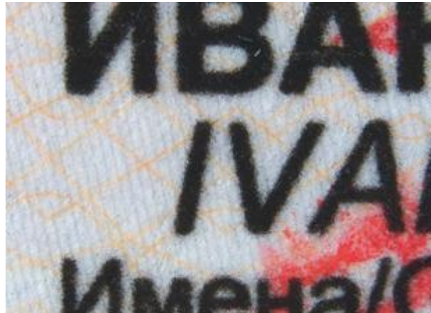
Biodata & photo integration technique: laser printing
