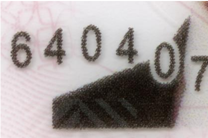
PCP® (Polycarbonate Colour Personalisation) technology
