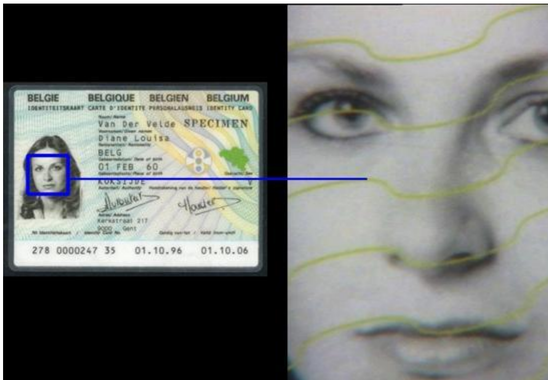
Biodata integration by photographic process
