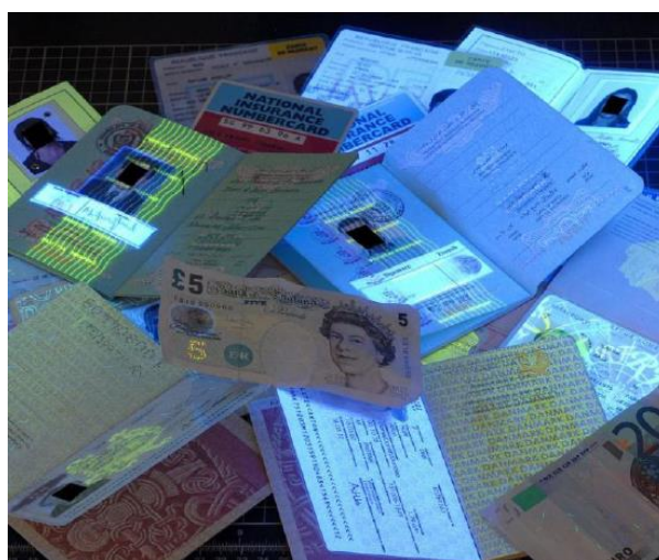
UV LIGHT: Counterfeit (parts of) documents fluoresce (shine) more brightly
