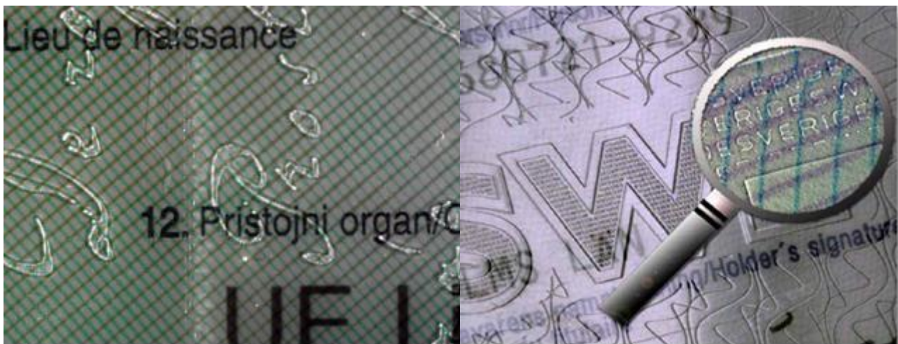
Laminate embossing with microprint
