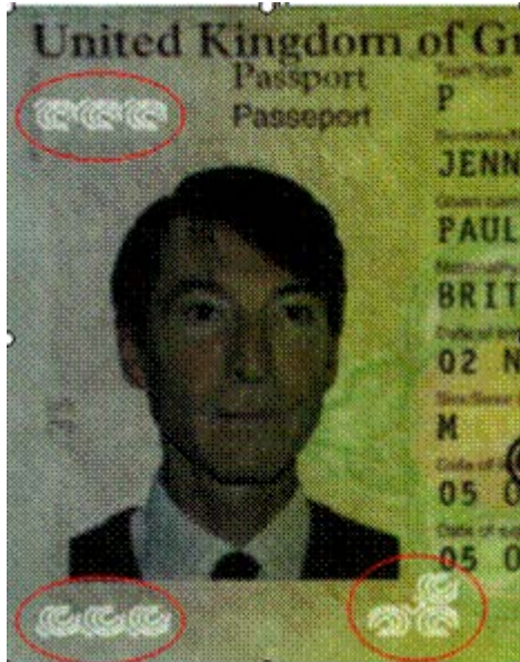
Laser-perforated structures/designs: Destri Perf®
