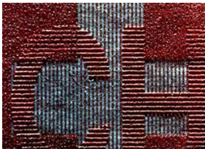
Line structure (90°) of the latent image
